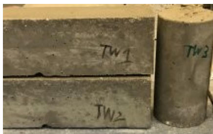
Figura 4 – Concreto com grafeno – Fonte: University of Exeter. 2018. Disponível em: https://www.exeter.ac.uk/news/research/title_654766_en.html acessado em: 18/11/19
